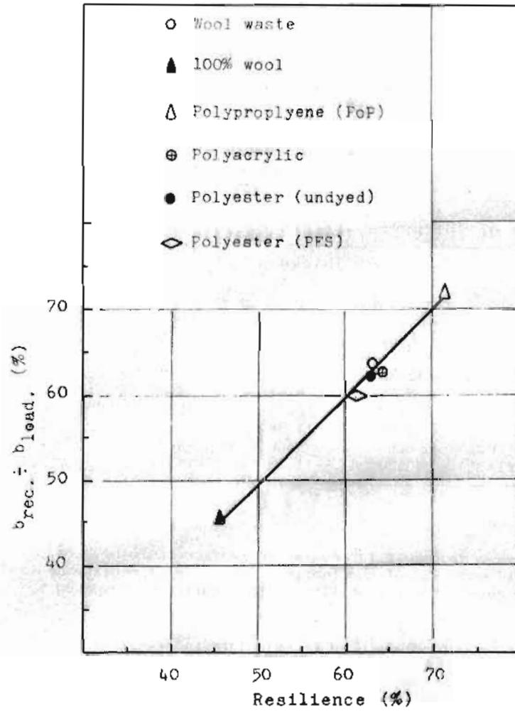
Fig.5 Values of  $b_{rec.} / b_{load.}$  Versus Resilience
