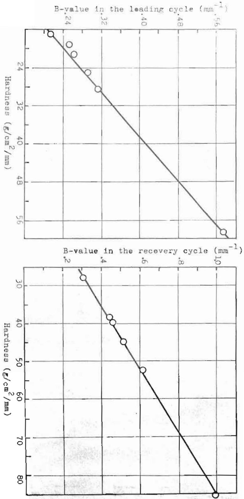
Fig.2 Fabric Final Incompressibility Coefficient(B)
