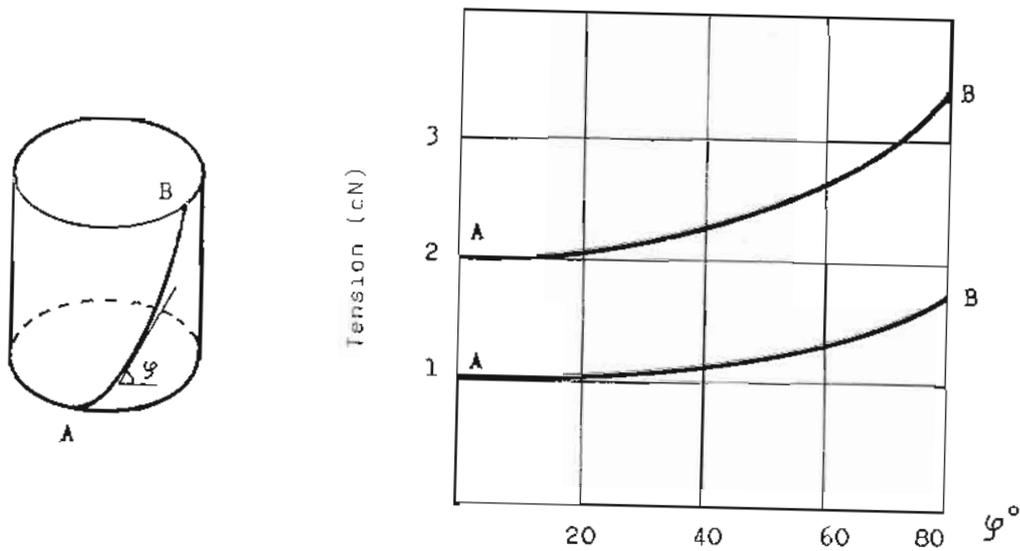
Fig. 3: Theoretical relationship between yarn tension and angle  $\psi$ .
