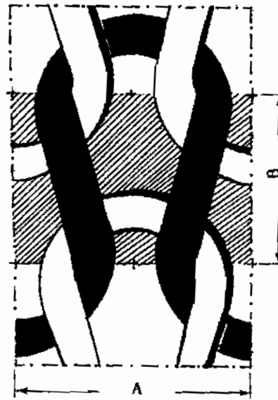
Fig. 1 Geometrical Model of Jersey Stitch
