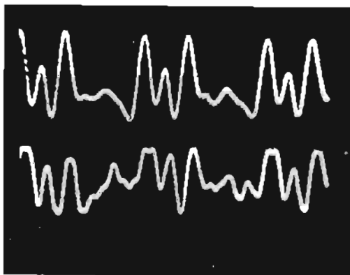
Fig. 24 a)Original Speech Signal b)Received Signal from 32Kbps System & SNR=10dB
