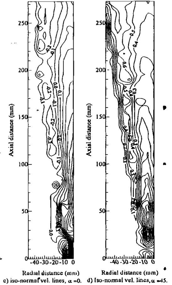
Fig. (10) Normal velocity in vertical diametric plane of swirl jet.
