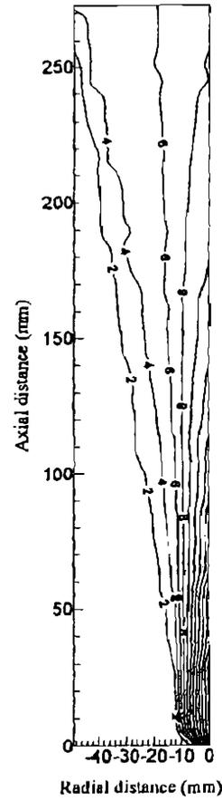
e) Iso-axial velocity line,  $\alpha = 0$  d) Iso-axial velocity line,  $\alpha = 45$
