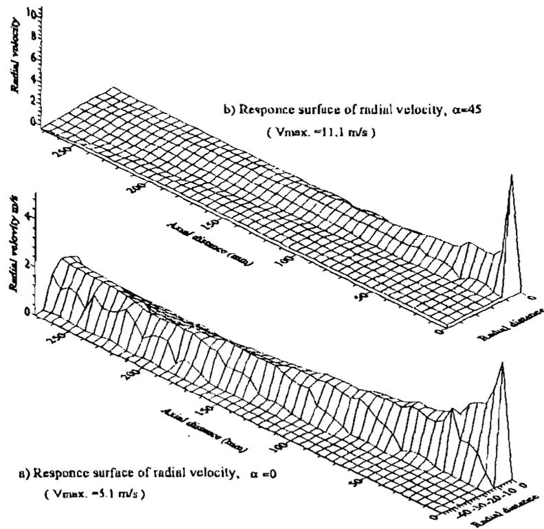
Fig. (9) The radial velocity component in vertical diametric plane of swirl jet.
