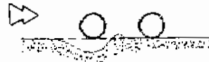
a) Scour under the first line only F = 0.18, y = 2.5\phi, S = 3\phi
