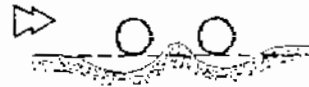
d) Wavy scour hole with an apex in between F = 0.19, y = 3\phi, S = 2\phi
