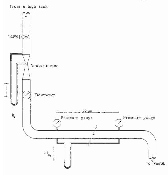
Fig(1) Experimental setup (schematic)
