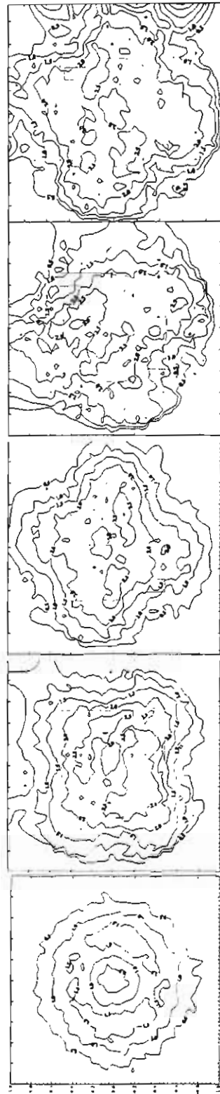
A1) Baseline jet (without inj.) A2) SJ \alpha=0^\circ mr=0.055 A3) SJ \alpha=45^\circ mr=0.055 A4) SJ \alpha=0^\circ mr=0.078 A5) SJ \alpha=45^\circ mr=0.078 Fig. 10 Experimental iso-contour of total turbulence kinetic energy [(u^2 + v^2 + w^2)/2] , ( m^2/s^2 ), for baseline jet and swirl jet at a horizontal plane.
