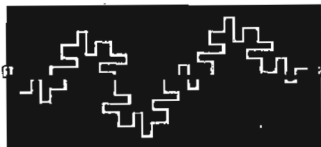
(b) Eight continuous Minkowski fractal slots (c) Twelve continuous Minkowski fractal slots Fig. 2. Minkowski fractal slots in ground plane
