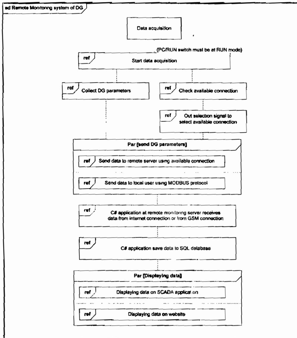
Figure 3 Remote monitoring system sequence diagram describes the sequence operation
