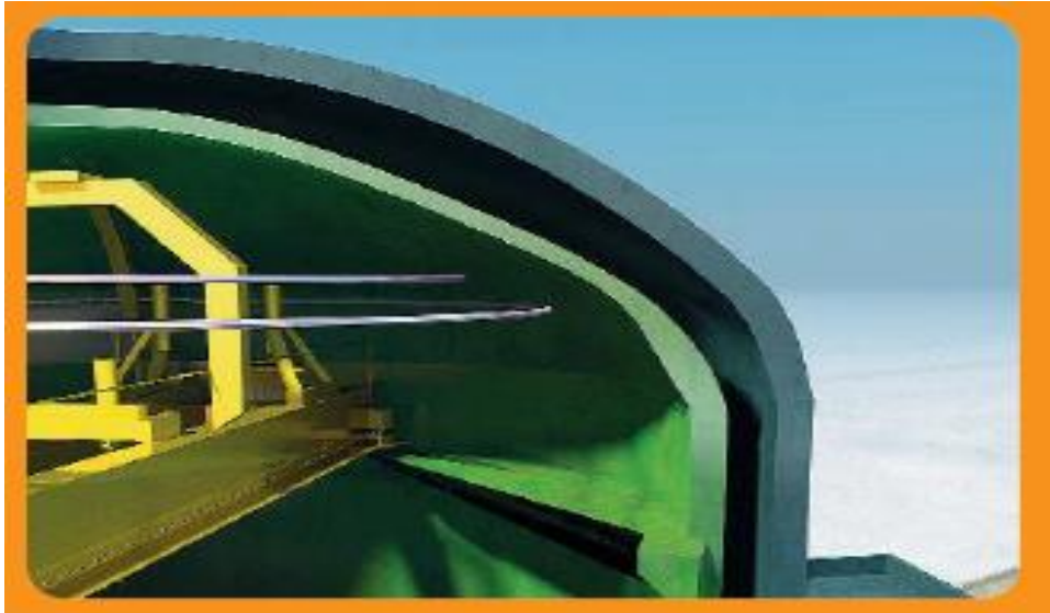
Fig. (1) Double wall of new generation of nuclear plants ( www.AREVA.com )
