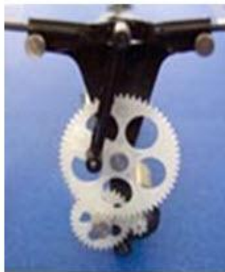
Fig.3. A simple Four bar flapping mechanism
