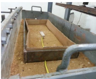
Figure 11. Strain Gages Under AC Layer
