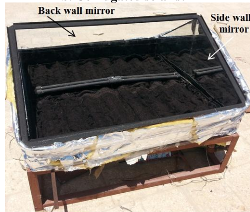
d. Corrugated still with wick and reflectors
