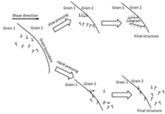
Fig. 8 Role of dislocation motion on the final grain size during different ram speeds
