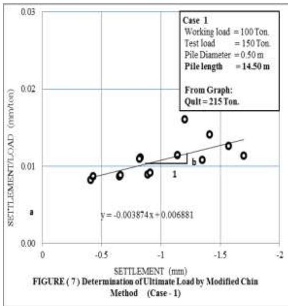
FIGURE ( 7 ) Determination of Ultimate Load by Modified Chin Method ( Case -1)
