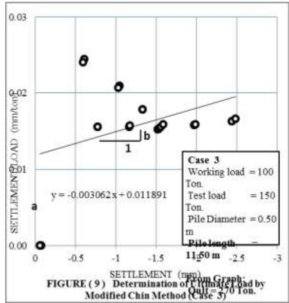
FIGURE ( 9 ) Determination of Ultimate Load by Modified Chin Method ( Case 5)
