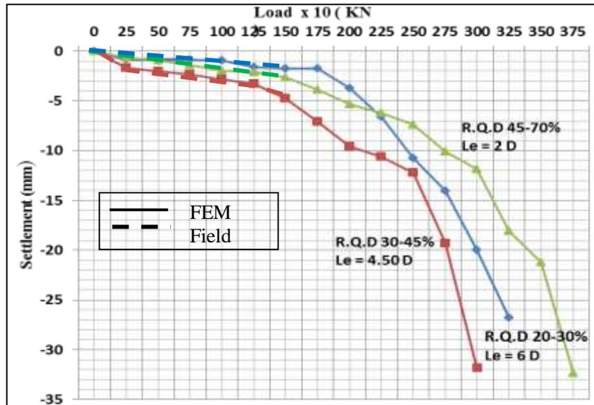
Figure (4) Results of FEM compared with the field load-settlement data
