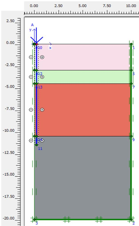
Figure (2) Geometry model of pile
