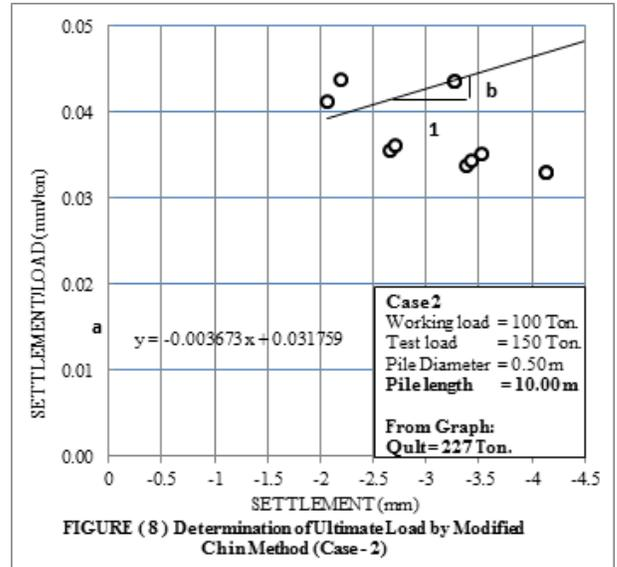
FIGURE ( 8 ) Determination of Ultimate Load by Modified Chin Method ( Case -2)
