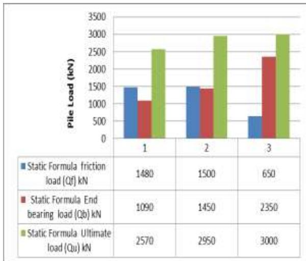
Figure (5) Friction and end bearing pile loads
