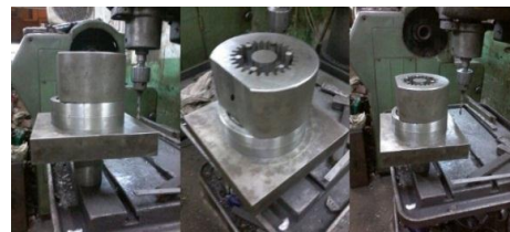
Figure.8 the die parts fixed on table
