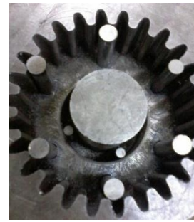
Figure.6 The die holes for ejectors
