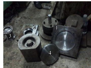
Figure.7 The die parts 1_base of die2_bearing holder 3_rod 4_Cover of Die
