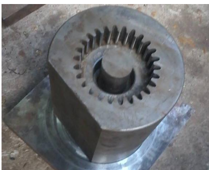
Figure.5 The die after milling
