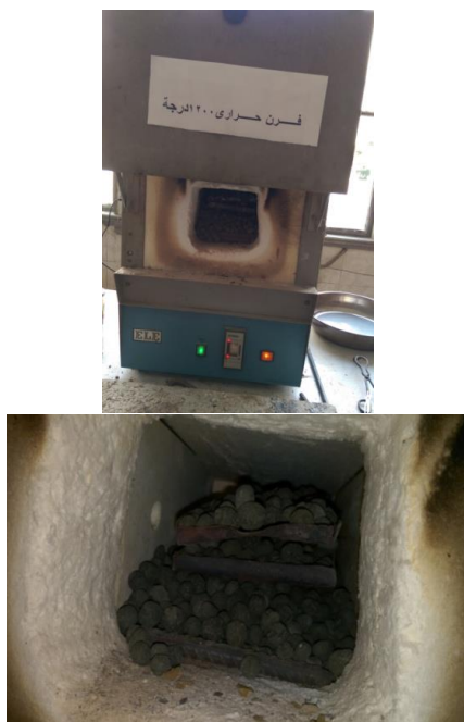
Figure (4): Firing up to (500 and 700) °C in furnace electric in concrete laboratory, faculty of engineering, Mansoura University
