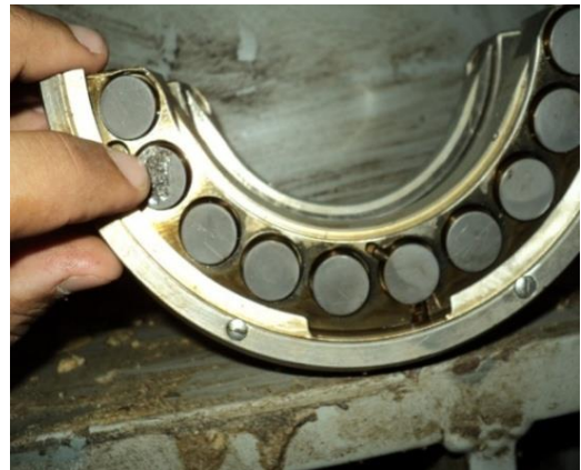
Fig.11. Defects at the thrust bearing pads
