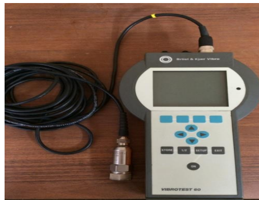
Fig. 3 Vibration data collector (B&amp;K VIBRO 60)
