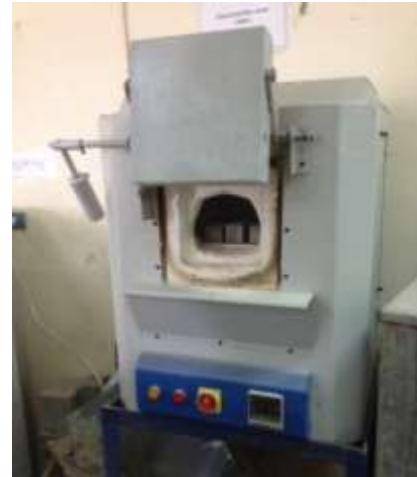
Fig. 4: Automatic electric furnace for elevated temperatures exposure
