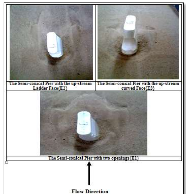
Figure 17. The lab images for the second set piers.
