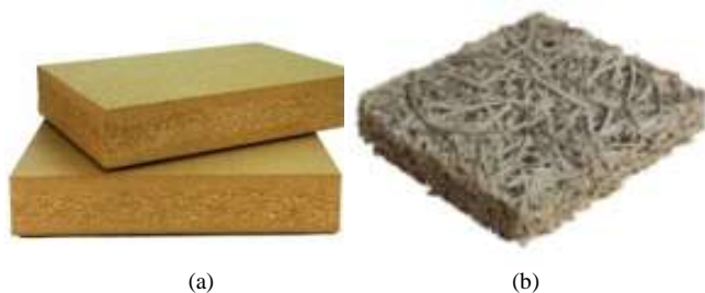
Fig. 10. Sustainable insulation material (a) Straw board (b) wood wool board.
