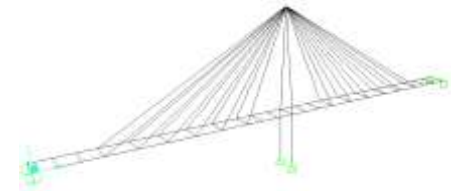
Fig.(6b): Radiating Bridge.
