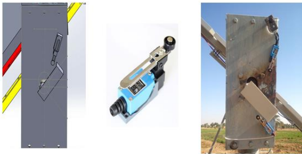
Fig.5. Limit switch used in the system
