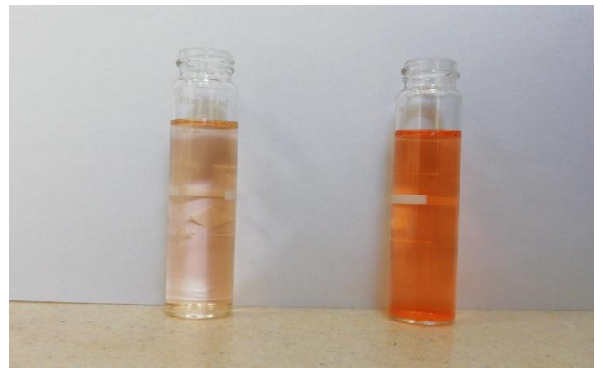
Photo2. Effect of contact time (CT): initial concentration 1.72 mg.l -1 and after 60 min=0.1 mg.l -1
