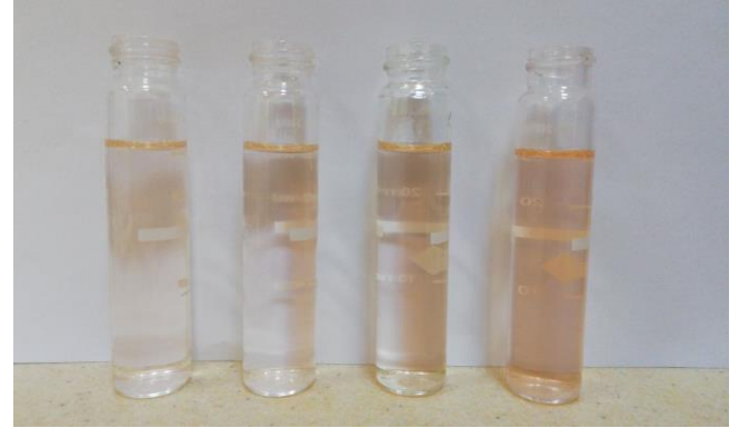
Photo1. Effect of contact time (CT) on iron removal by FHA200, after 15,30,45,60 min
