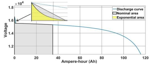
Fig. 10. The characteristics of the lead-acid battery [24].
