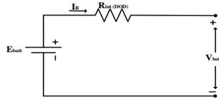
Fig. 9. Equivalent circuit of battery [24].
