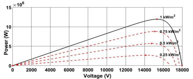
Fig. 4. (P-V) features of a photovoltaic system [25].
