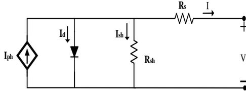
Fig. 2. The equivalent circuit of solar cell.
