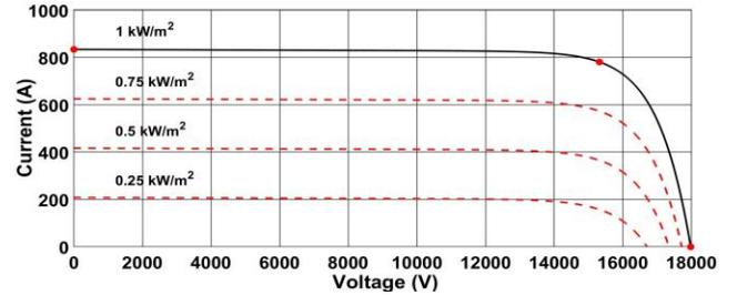
Fig. 3. I-V features of a photovoltaic system [25].
