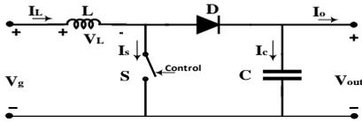
Fig. 5. Equivalent circuit of the boost converter.
