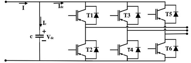
Fig. 8. Equivalent circuit of the VSC [27].
