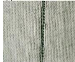
Fig. 1: Laddering defect in knitted fabrics
