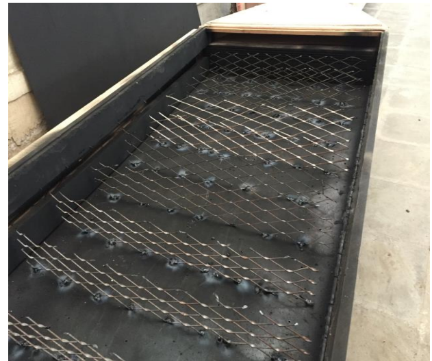
Fig. 4. Photo of wire-mesh position in the collector.
