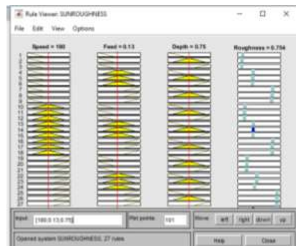
Fig. 12 (b) Viewer of FIS rule for Ra prediction by the second method.
