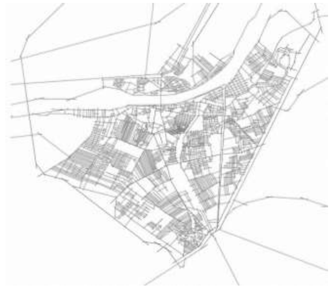
Fig. 5. Axial Map, Spatial representation of Mansoura city. Source: The Authors, using Auto Cad software overlaying the Open Street Map. Date: April 2020
