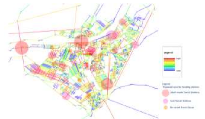
Fig. 7. Integration measure analysis at local scale, using angular step measure where r=5 steps. Source: The Authors, using Depthmap software. April 2020
