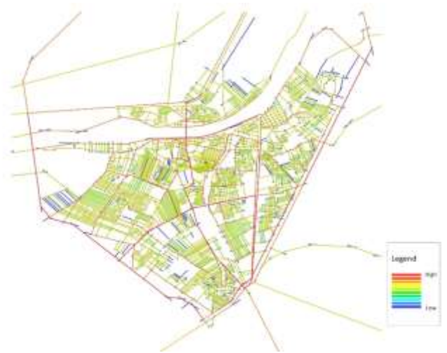
Fig. 6. Normalized Choice analysis at global scale where r=n . Source: The Authors, using Depthmap software. Date: April 2020
