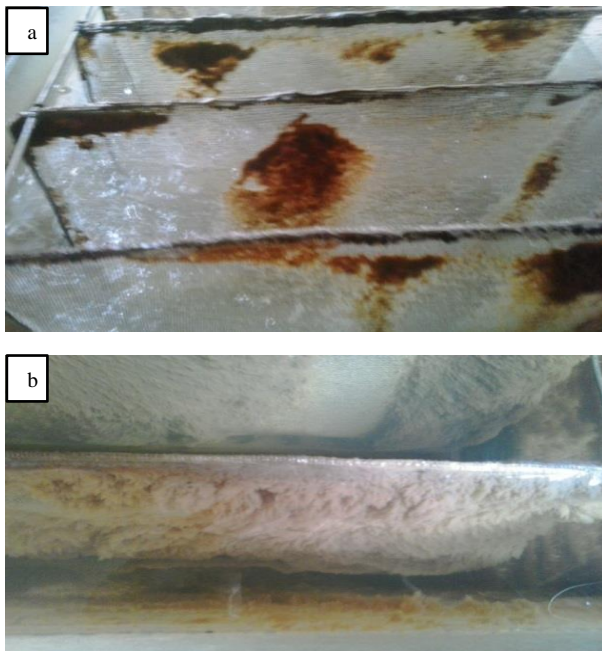
Fig.2. Shown the surface of media (a) after 5 days startup (b) after 30 days of start-up
