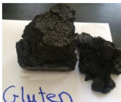
Fig. 8. Failure of Bitumen and Gluten Specimens due to water absorption.
