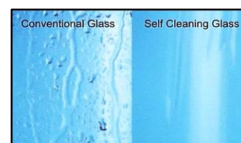
Fig. 3. Comparison of conventional and self-cleaning glasses. (adapted from Pro Clean Window 2018) [12].
