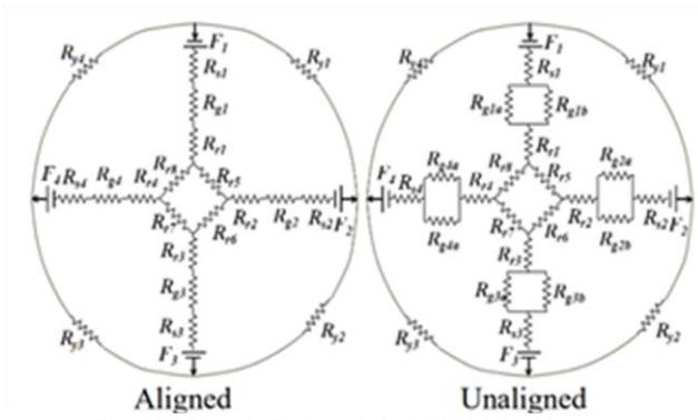
Fig. 16. Magnetic flux's path for RFSRM; healthy case
