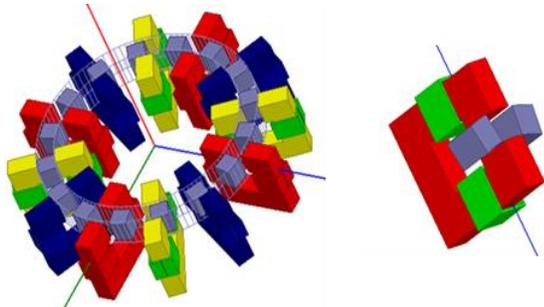
Fig. 7. 3D FEM geometric of 12/16 C-Core SRM
