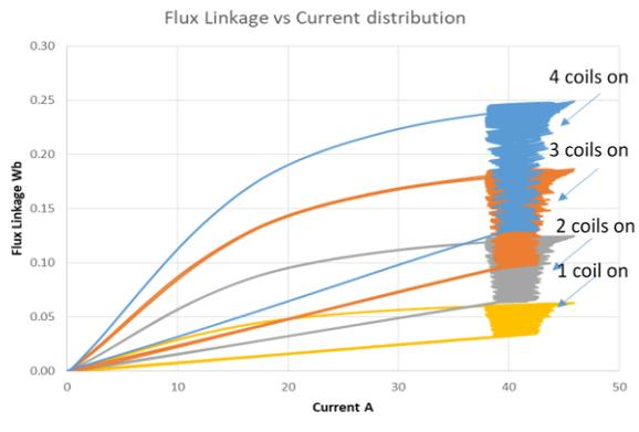
Fig. ٧. Flux linkage / current distribution
