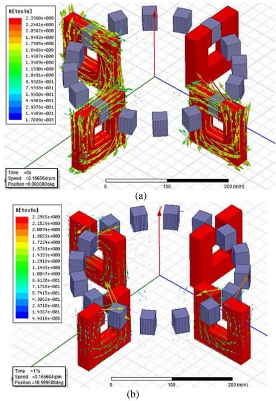
Fig. 11. 3D flux density distribution for 3 healthy coils and 1 faulty coil; (a) aligned and (b) unaligned position
