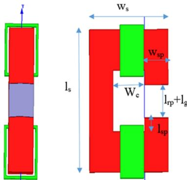
Fig. 8. 2D geometric of C-Core SRM single segment
