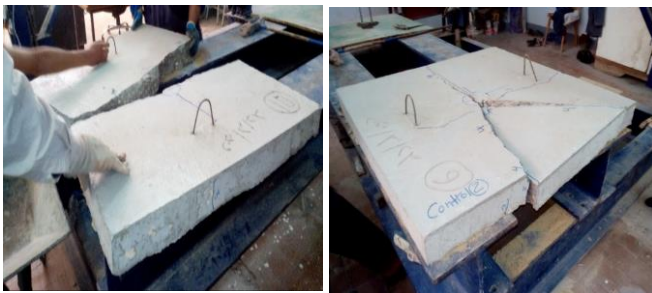
Figure 7. The control slab (CR 0) -Top surface
