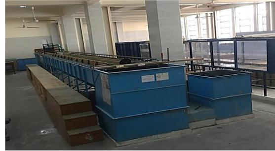
Photo (1): The experimental flume.
