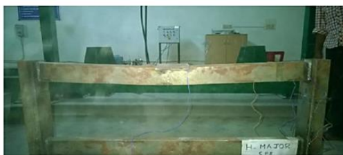
failure in major axis
