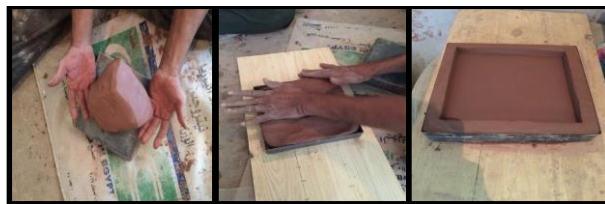
Photo (1): Forming the membranes filter shape
