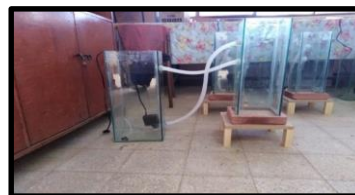
Photo (2): Experimental set-up for filtration tests.
