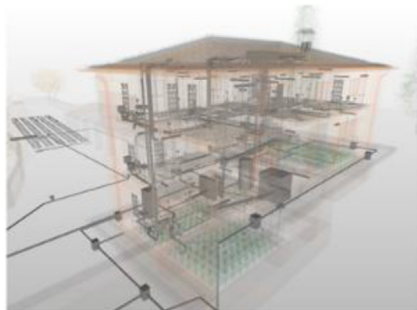
Fig. 8. 3D view of the multidisciplinary (Mechanical–Electrical–Plumbing (MEP) model (Piselli, 2020a, b).
