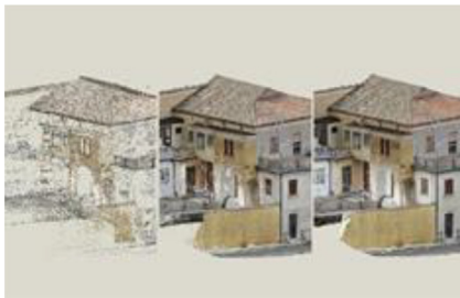
Fig. 6. Laser scanner survey Ref. Piselli (Piselli, 2020a, b).
