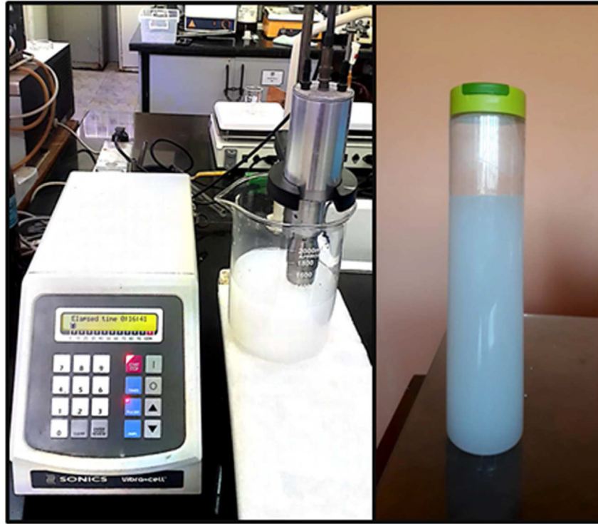
Fig. 4. Nanofluid preparation using ultrasonic liquid processor.
