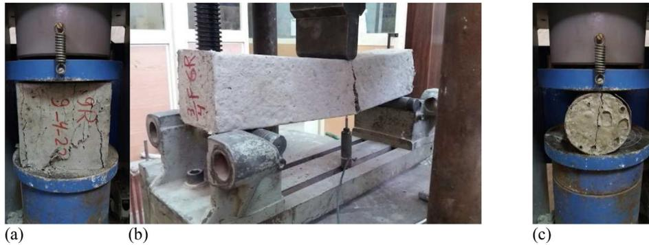
Fig. 3. Mechanical properties tests of concrete samples (a) Compressive strength test, (b) Flexural strength test, and (c) Splitting strength test.
