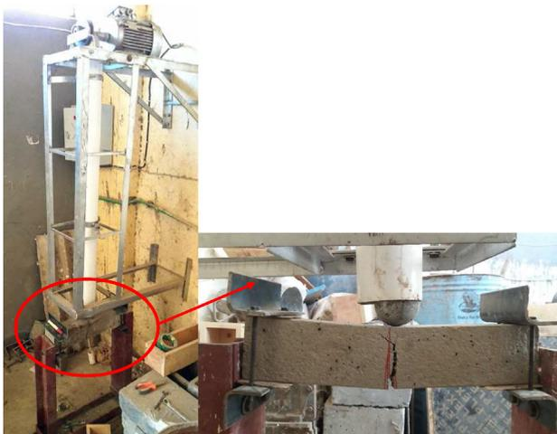
Fig. 4. The impact resistance under flexural load test.
