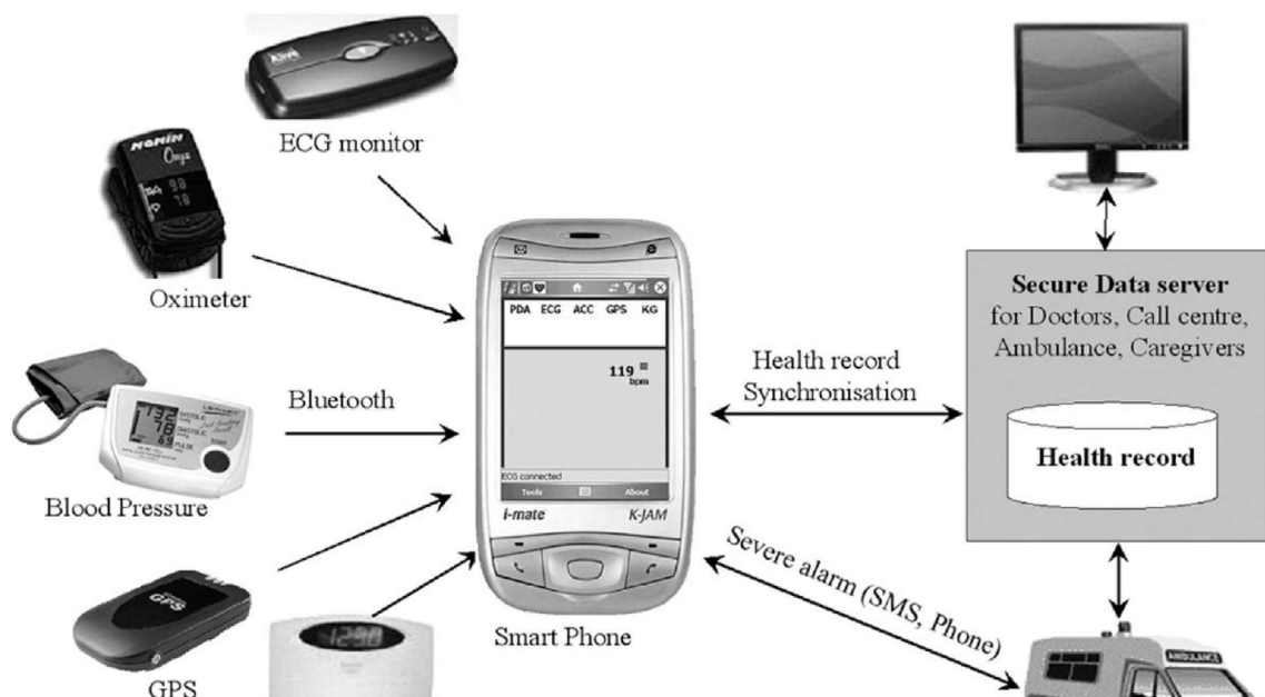
Fig. 1. Heart-monitoring system architecture (Leijdekkers, 2007).
