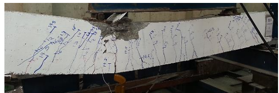
Fig. 11 Crack pattern of Beam BS03
