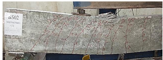
Fig. 9 Crack pattern of Beam BS02
