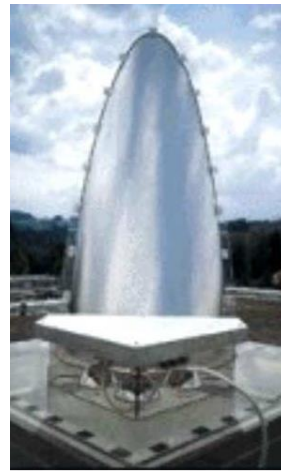
concave collector, Heliobus system in Switzerland
