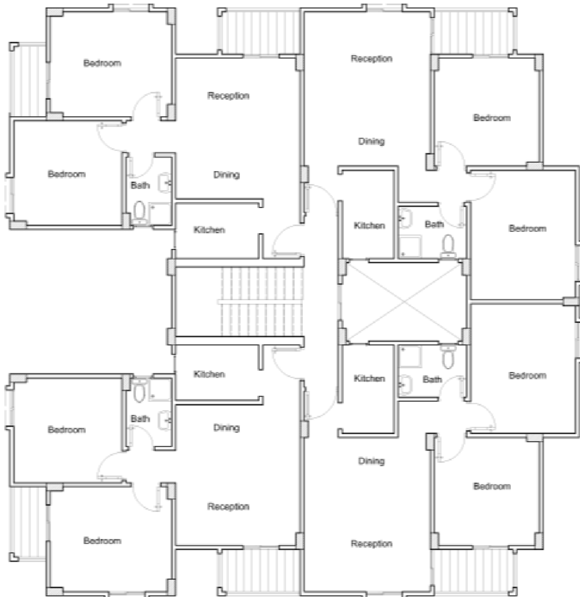
Fig. 11. The residential typical floor, youth dwelling, four units, staircase location, and service courtyard.
