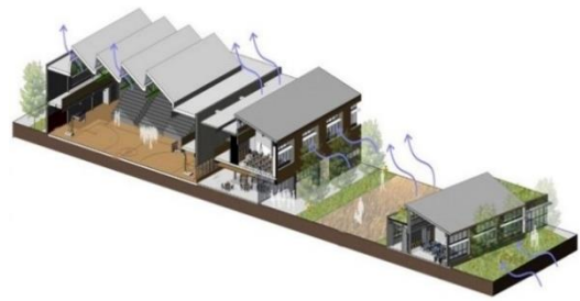
Figure 5: Greensburg make use of the prevailing breezes in the strategy. (AIA, 2011)
