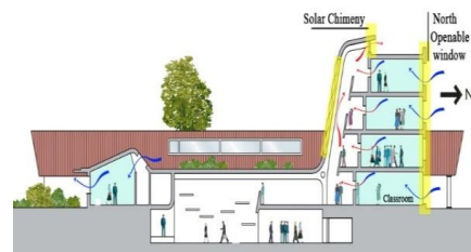
Figure 9: The north storey teaching block with a south-facing solar atrium is prominently positioned act as solar chimney. (Britain, 2006)
