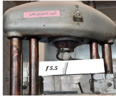
(b) Beam with PO fiber 5.5
