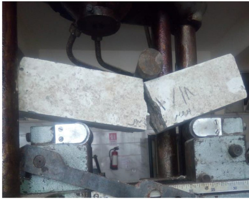
(a) Beam with PO fiber 00
