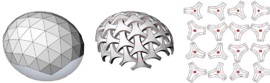
Fig. 12. Grid Modelling, assigning components with curved line folding and extraction of component's fabrication data in flat state are the steps applied in digital tools (Brancart et al., 2015).
