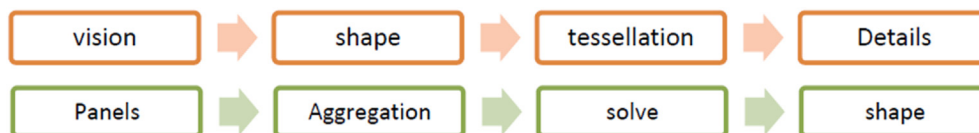
Fig. 3. Design approaches (Top) top-down steps flowchart (bottom) bottom-up steps flowchart.
