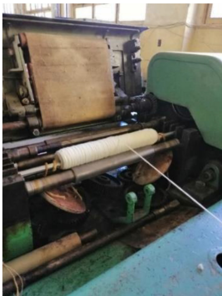
Fig. 2. Winding the roving on the perforated pipe.
