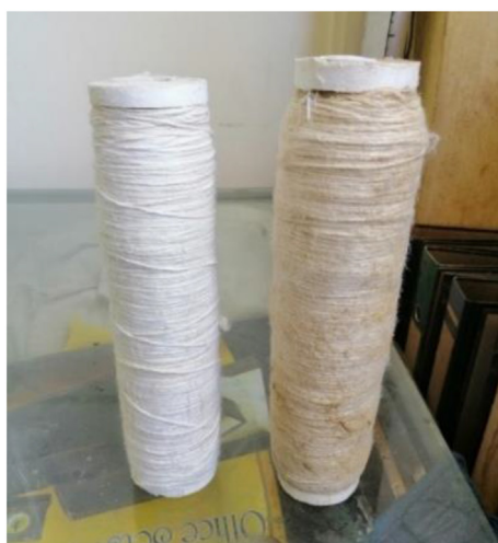
Fig. 8. The shape of the filter candle before and after filtration.
